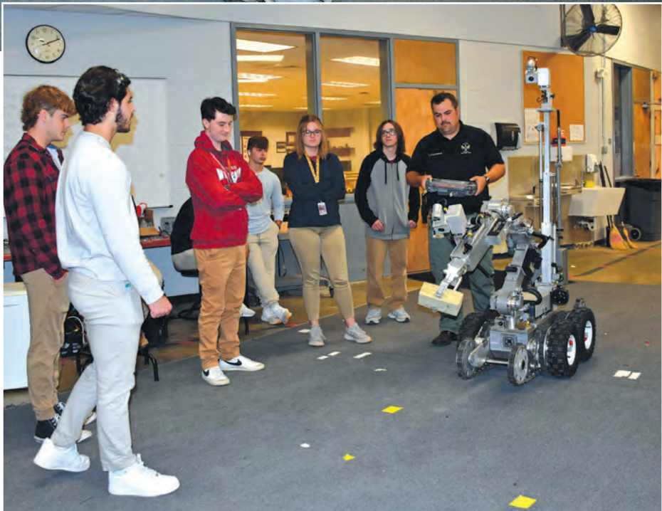
The SRT robot is used in situations where a police officer cannot access an area safely.
